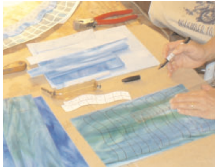
2. Patterns are arranged onto sheet glass and cut.
