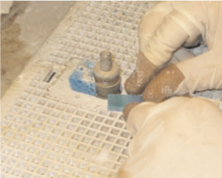
3. Each piece is grinded to remove sharp edges.
