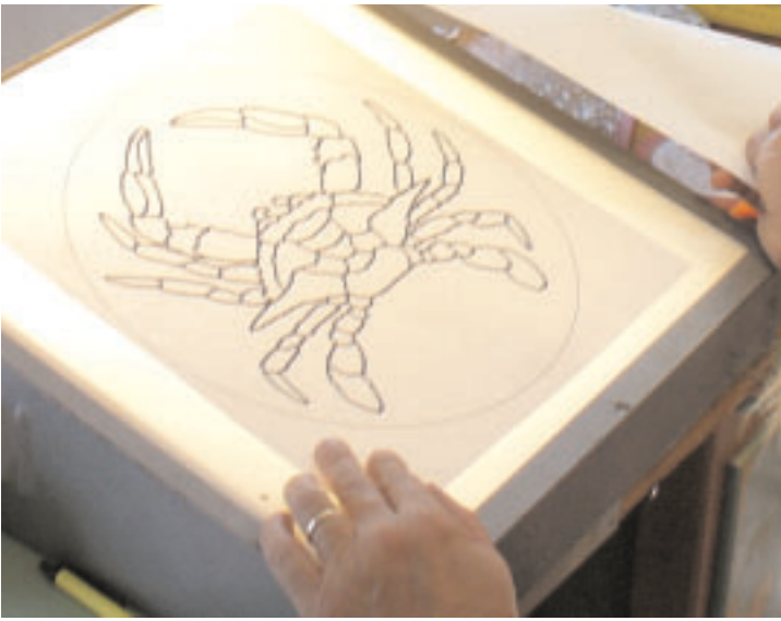
1. Once the design is done, a template is made.
